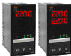
Outline dimension: 80×160×115mm Open hole dimension: 76^{+0.7}_{-0} \times 152^{+0.7}_{-0} mm
